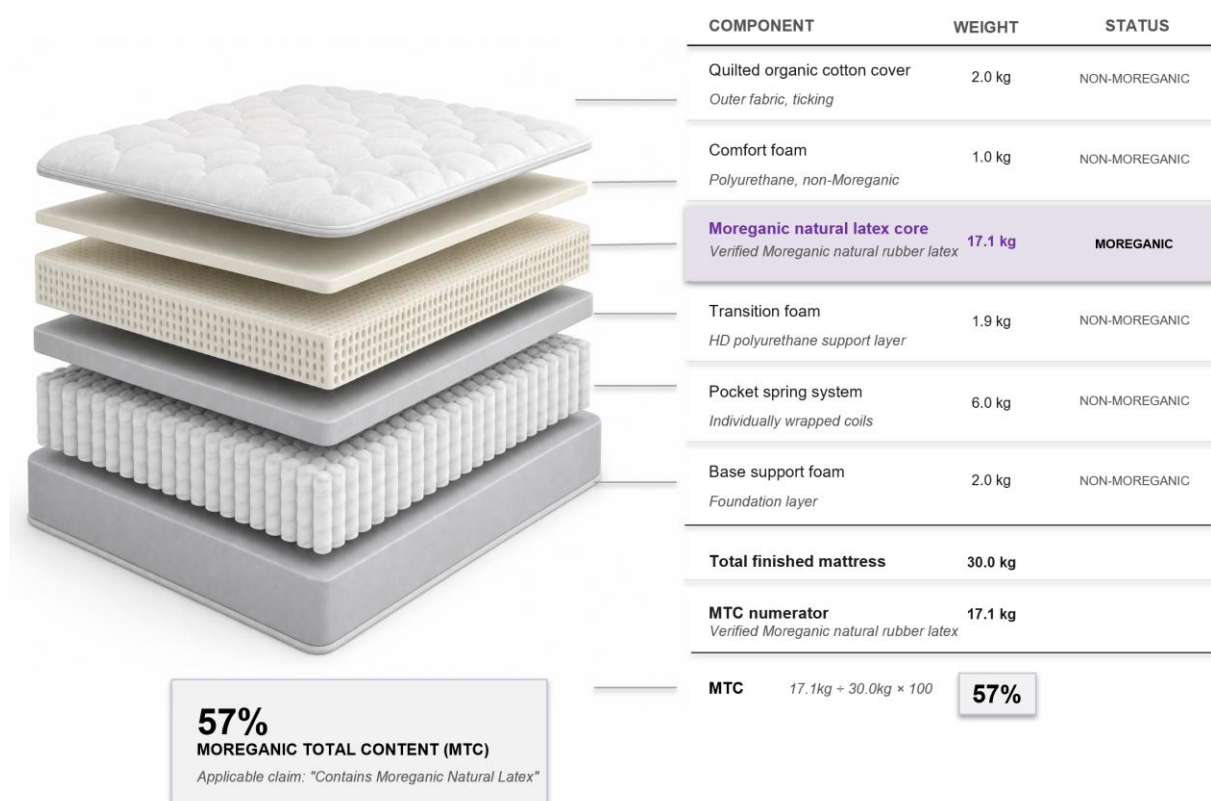
Figure 1 Illustrative finished mattress structure. The Moreganic natural latex core is the only Moreganic component. All layers are included in the total finished product weight, while only the verified Moreganic natural rubber latex enters the MTC numerator.
